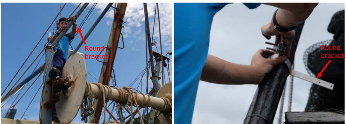
Figure 4. Jonathan (MRF) installing the round bracket on a fishing trawler.
