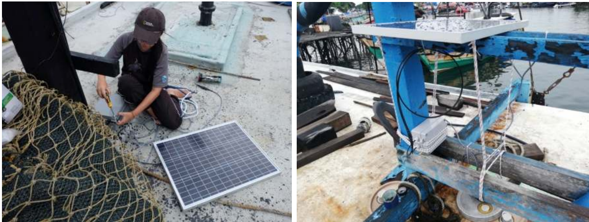
Figure 3. KC (MRF) installing the solar panel and the battery on a trawler.
