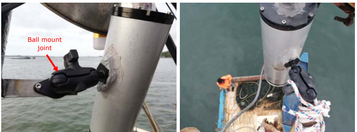
Figure 5. The electronic monitoring camera is attached to the round bracket using a ball mount joint.
