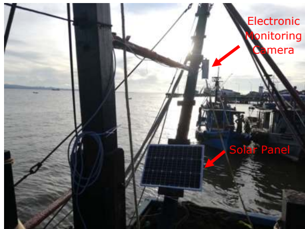
Figure 7. The complete installed electronic monitoring camera on a fish trawler. Images are downloaded when the trawler comes back from the sea.
