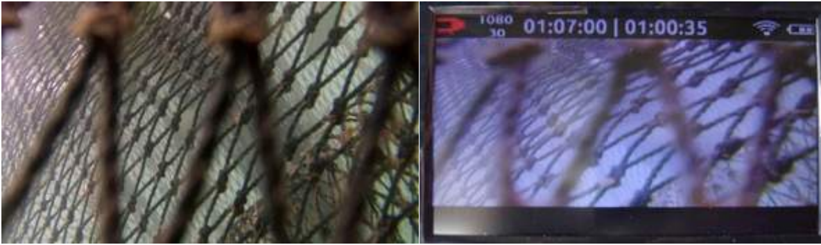
Figure 2-9: Comparison between the screenshots of the footage obtained by the GoPro recording at 10m depth and ~ 200m behind the vessel and the same time stamp on the video screen on the vessel.
